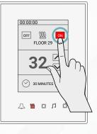
**3** Test the floor heating by changing the temperature and turning it OFF/ON.
