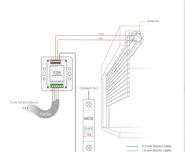
Figure 2: TIT-3G-BUS-S & Motors Connection Diagram
