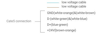
Figure 5: TIT-3G-Bus-S & Traditional Switch Connection Diagram
