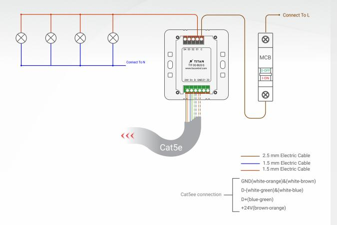
Figure 1: TIT-3G-BUS-S & Lights Connection Diagram
