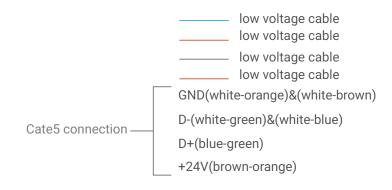
Figure 4: TIT-3G-Bus-S & 3rd Party Sensor Connection Diagram
