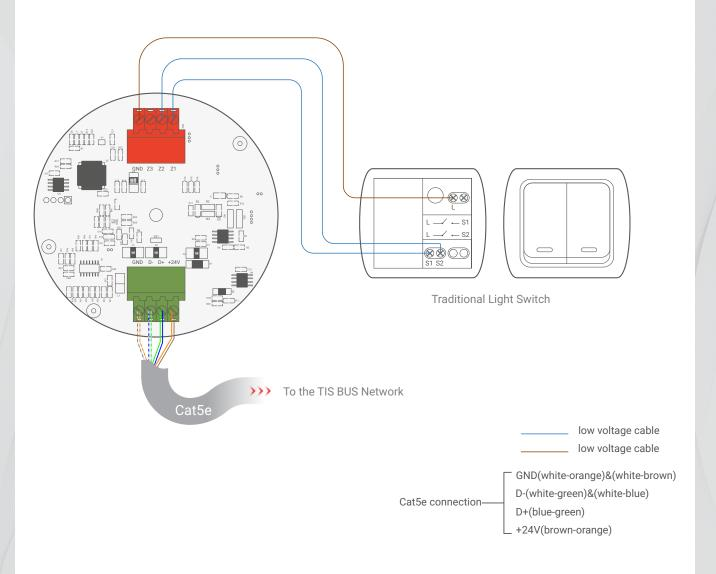
Figure 2: Traditional Light Switch Connection Diagram
