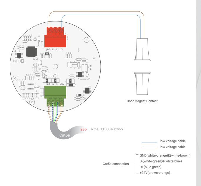
**Figure 3: Magnetic Door Contact Connection Diagram**
