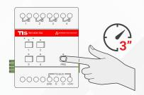
Short press on the first button and then **2** the second button that you want to combine as curtain control; for example, CH3 and CH4.
