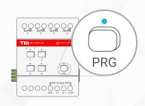
Test by turning the first button ON and 4 then the second button. Both buttons should not turn ON together. If you see that the first button is turning the other button off, that means that your buttons are successfully combined as shutter/ curtain mode.
