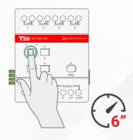
Go to floor heater page on any wall panel with the floor heating function, and press ON button to turn on the floor heating.
