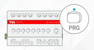
Test by turning the first button ON and 4 >>> then the second button. Both buttons should not turn ON together. If you see that the first button is turning the other button off, that means that your buttons are successfully combined as shutter/ curtain mode.
