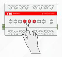
Wait for a few seconds until the PRG LED stops blinking.
