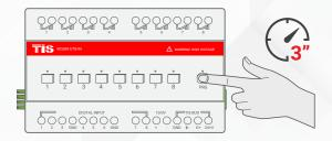
Short press on the first button and then **2** the second button that you want to combine as curtain control; for example, CH3 and CH4.
