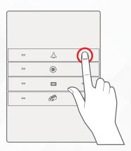
Test the button on the panel by short **3** pressing it for ON/OFF and long pressing it to dim (if channel is dimmable).
