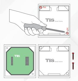
Connect the Wall Base and Panel 4>> Addition in this position. Place the upper pins as shown, and then push the down pins down with your fingers to assemble.
