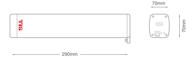
**Figure 2: Module Dimensions**
