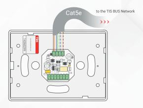
Connect the other connection if needed **5** between wall services switches to the digital inputs of the hotel panel as per the following diagram.
