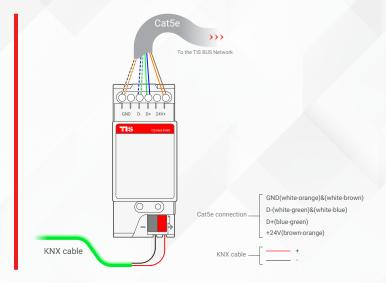
Turn on TIS power supply and KNX **5**>> Power supply, The module's PRG green LED should start blinking.
