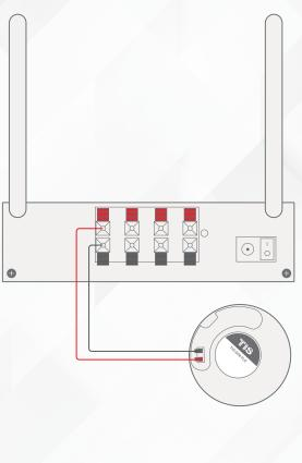
2 Link the Bus cable to TIS-BUS network in case of operating the Matrix in 2-4 separated audio zones.
