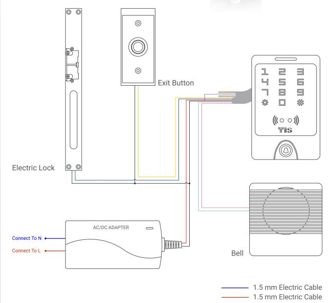
▲ Figure 1: TIS Access Control Wiring Diagram
