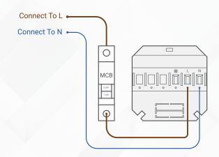
7 ➤ Attach the load wire to the ⊗ terminal.
