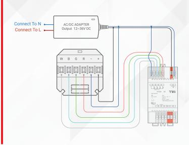
Connect the LED lights wires to the 0-10V driver.
