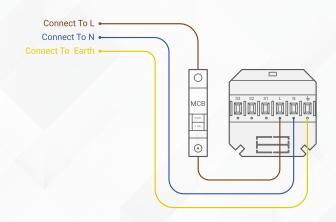
**7** Attach the switch1, 2, & 3 wires to the S1, S2, & S3 terminals, respectively.
