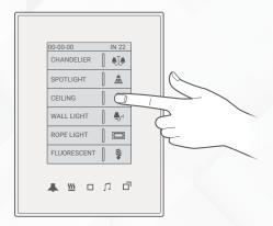
Test by pressing on the wall panel's ON/ **3** OFF button. The module should respond by turning ON and OFF accordingly.
