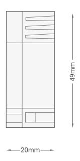
Figure 6: Module's Dimensions
