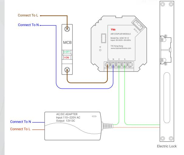
low voltage cable low voltage cable 2.5 mm Electric Cable — 1.5 mm Electric Cable 1.5 mm Electric Cable
