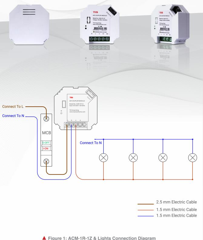
▲ Figure 1: ACM-1R-1Z & Lights Connection Diagram
