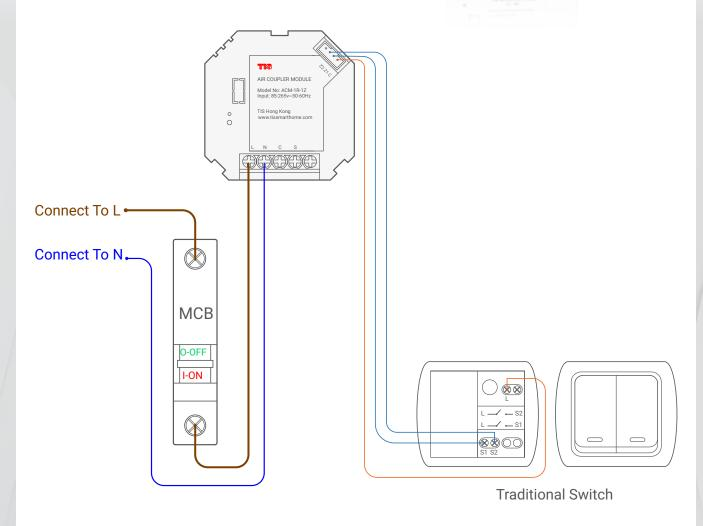
Figure 5: ACM-1R-1Z & Traditional Switch Connection Diagram
