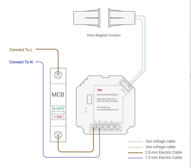
Figure 4: ACM-1R-1Z & Magnetic Door Contact Connection Diagram
