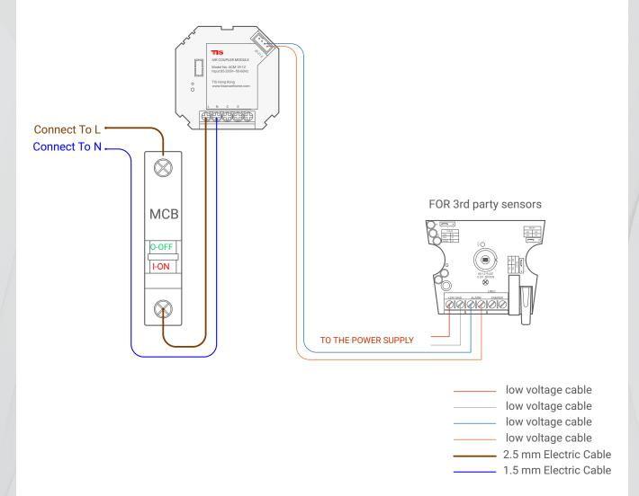
Figure 3: ACM-1R-1Z & 3rd Party Sensor Connection Diagram
